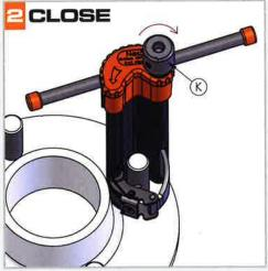
(B). Place Nes5 over thread to be repaired. grooves of thread, and tighten by hand only. direction of the arrow only.
