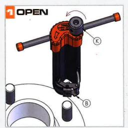
Turn knob (K) to expand the blades' carrier Turn knob (K) to move the blades into
